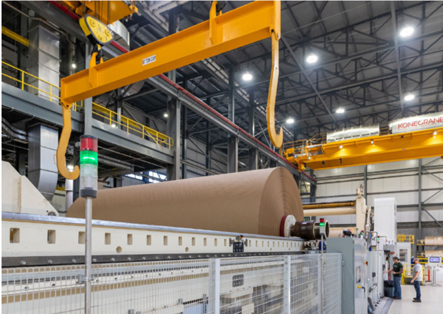
📷 Figure 2. An overhead crane — positioned by a PowerFlex drive — moves a roll of new paper for processing and printing.
